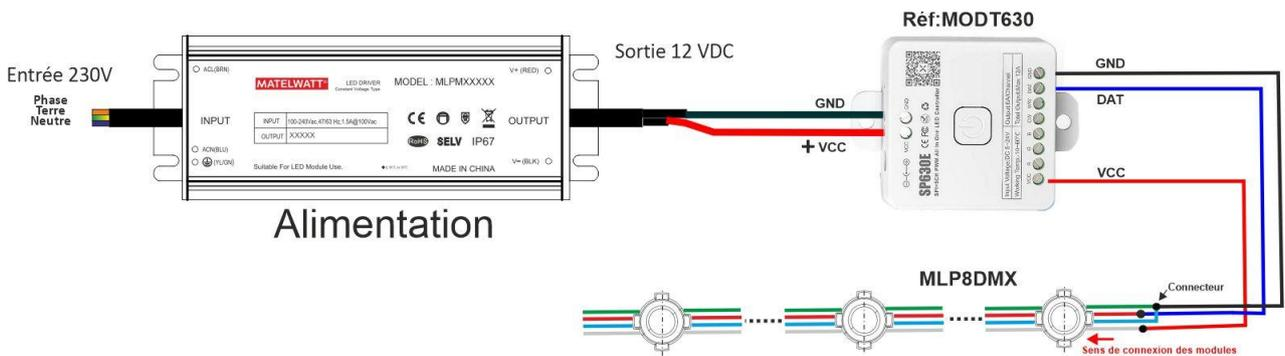
**CABLAGE AVEC INTERFACE DMX PROGRAMMABLE**
